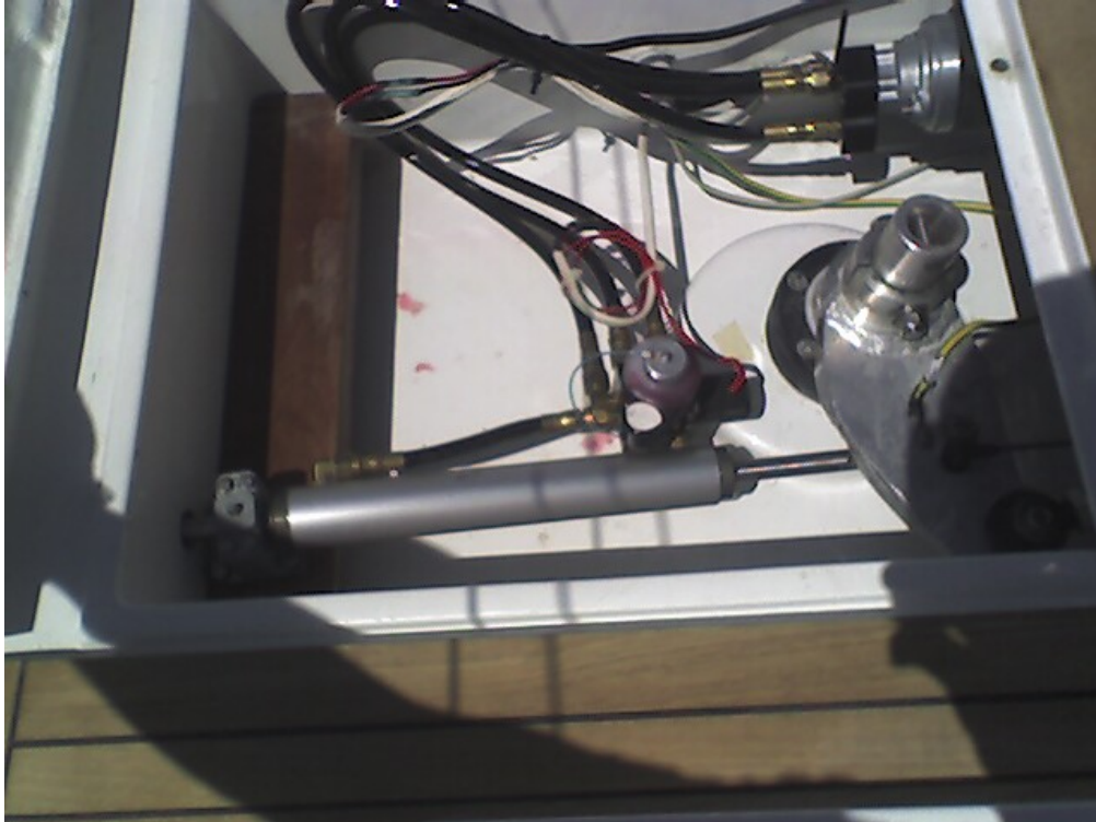
A Hanse 375 fitted with the versatile Octopus Linear Hydraulic drive unit
