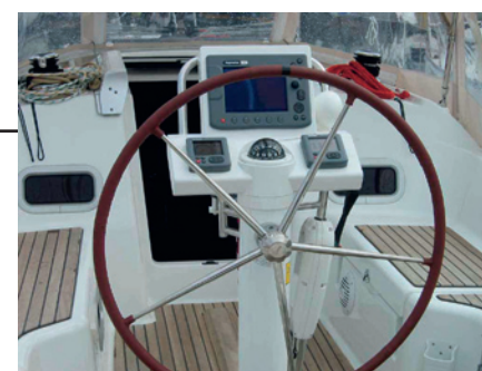
David's Raymarine system. The pilot display is the starboard instrument at the binnacle
